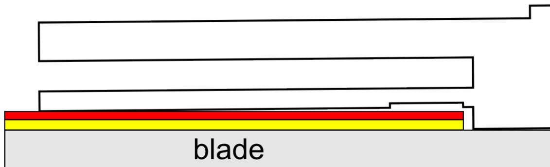
Rest the flat surface of the net gauge (left side in the pictures) on the rubber. If the 4mm protrusion (right side) touches the blade as in the picture above, then the racket covering is less than 4mm.
