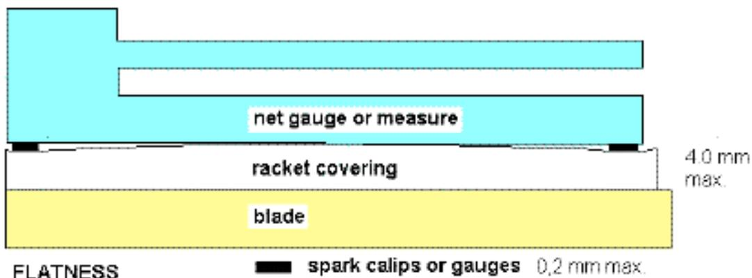
The magnitude of curvature can be tested by using standardized steel blades. In the picture above, the net gauge rests on 0.2mm blades. If the center of the net gauge touches the rubber surface, this indicates that this side of the racket is convex.
