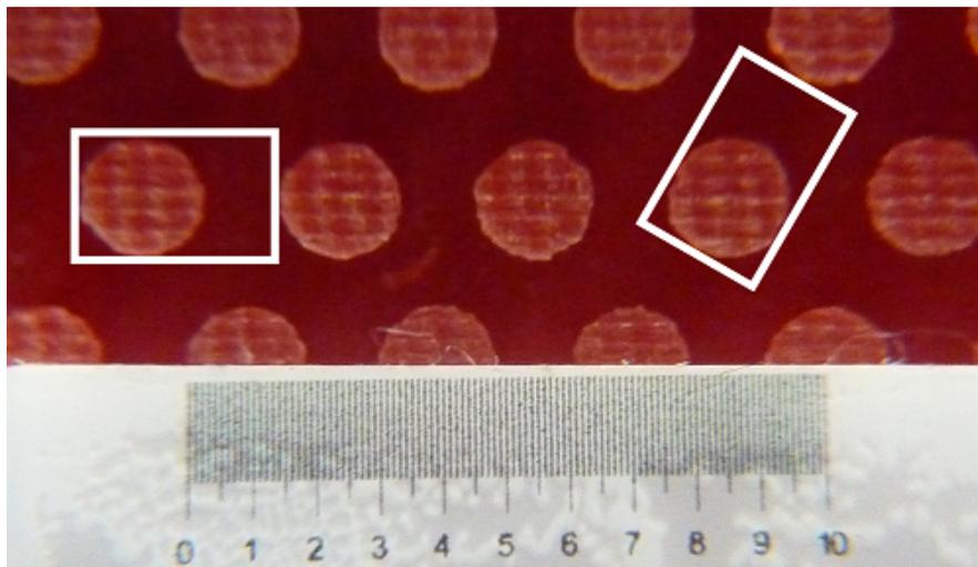
Measure the pimple spacing, defined as the diameter of an individual pimple plus the space to a neighboring pimple, shown with the white boxes above. (In this example the pimple spacing is approximately 3.0mm.)
